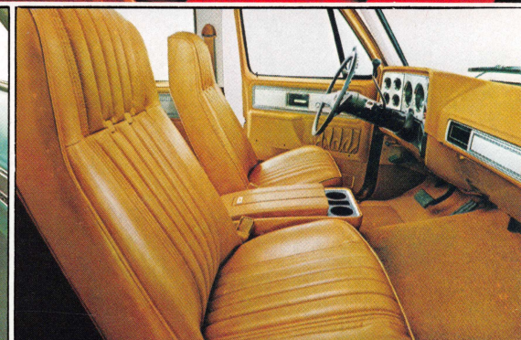
High-back bucket seats. Available with Silverado trim, Suburban's high-back buckets feature full-foam seat construction on a rugged steel frame for good support. Driver's seat is adjustable fore and aft to permit a choice of driving positions. Available options shown.
